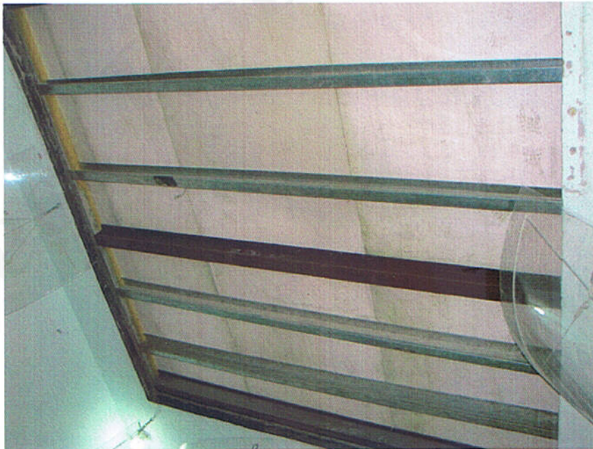
Figure 3 : Test setup of the "Besta" board panel system (underside) facing the receiving room
